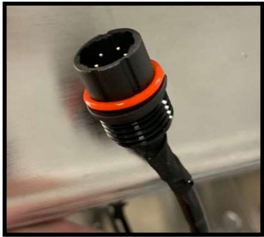
2. Connect the load cell to the male connector as shown in the chart that follows. Note that the male connector is mirror-image of the female one shown previously. The right side of the chart indicates the typical color codes for most load cells. Contact Hardy Technical Support at (858) 278-2900 Option #4 for assistance if your load cell differs.
